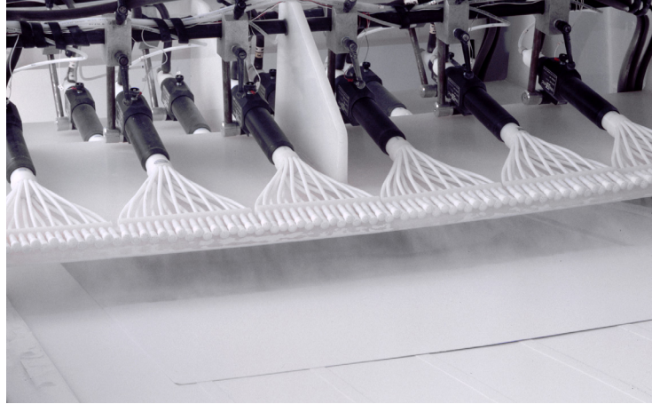
Nordson® Tribomatic® II automatic spray guns provide efficient part coverage at high line speeds.
